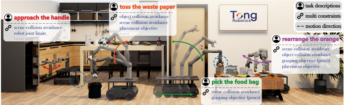
Fig. 1. Challenges in mobile manipulation. Mobile manipulation plays a pivotal role in core robotic tasks such as object grasping, placement, rearrangement, and articulated object manipulation. Each of these tasks poses distinct challenges, requiring the motion generator to holistically account for constraints posed by environmental geometry and robot embodiment to accomplish task-specific objectives.
